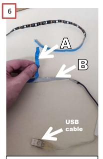
Unwind and remove light strip from spool. A) Remove blue backing from light strip. B) White adhesive will remain on light strip.
