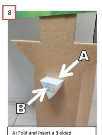
connector into the slots on the lower front of easel.
