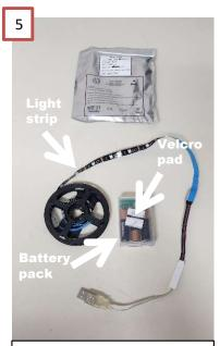
Unpack the light strip and battery pack from bag. Insert 3 AA batteries in battery pack. Attach one side of Velcro pad to battery pack cover.
